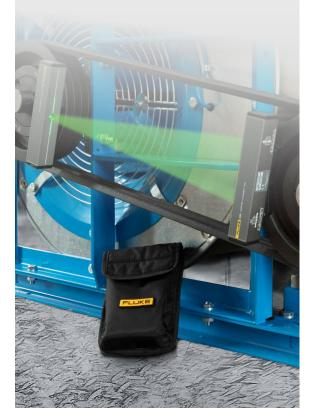
It's a known fact—all rotating machinery are susceptible to misalignment. An aligned pulley system reduces belt wear, power losses, and vibration of machinery, leading to improved performance.
