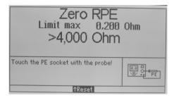
This menu makes it possible to balance the probe cable's resistance value.
