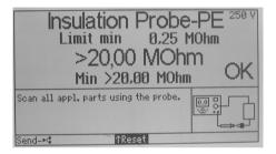
Insulation Resistance Measurement, Probe to Conductive Parts (which are connected to PE)
