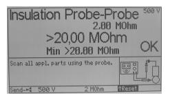
This measurement is intended exclusively for protection class III DUTs.
