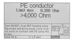
When the DUT is connected, resistance is measured between the protective conductor terminal at the test socket and the probe connection at the DUT (contact with conductive parts of the housing).
