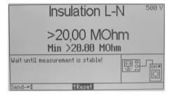
This measurement is used to test the insulation of, for example, extension cords and multiple outlets (via optional adapters) without circuitry (e.g. glow lamps).
