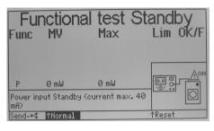
Current values of up to 40 mA can be measured for the display of small power values (mW range) in standby mode (DUT switched off).
