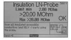
L and N are short-circuited in the test instrument during this measurement and a test voltage of 500 V (or 250 V with "Surge Arrester: Yes") is applied between LN and PF
