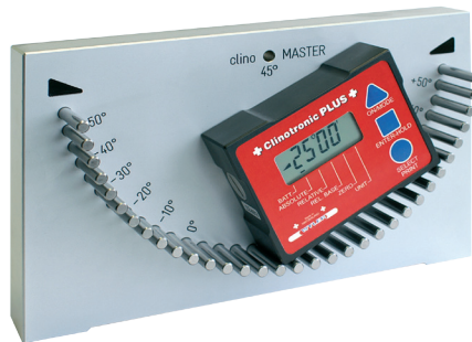
Version cast iron, surface chromium-plated
