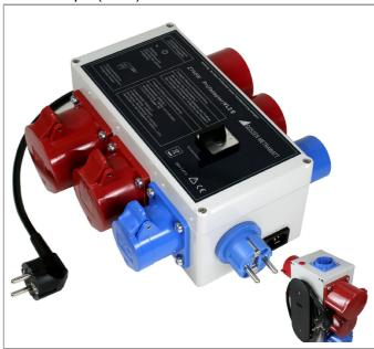
The test adapter is laid out for measuring and testing electrical devices and extension cables with CEE plug connectors in combination with test instruments, and is equipped to this end with single and 3-phase plug connectors up to CEE 32A.
